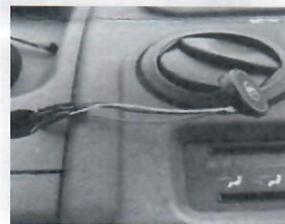
Connect the new changeover switch part no. DE802126.
