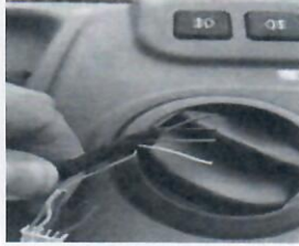
Cut and remove 5-pin connector.
